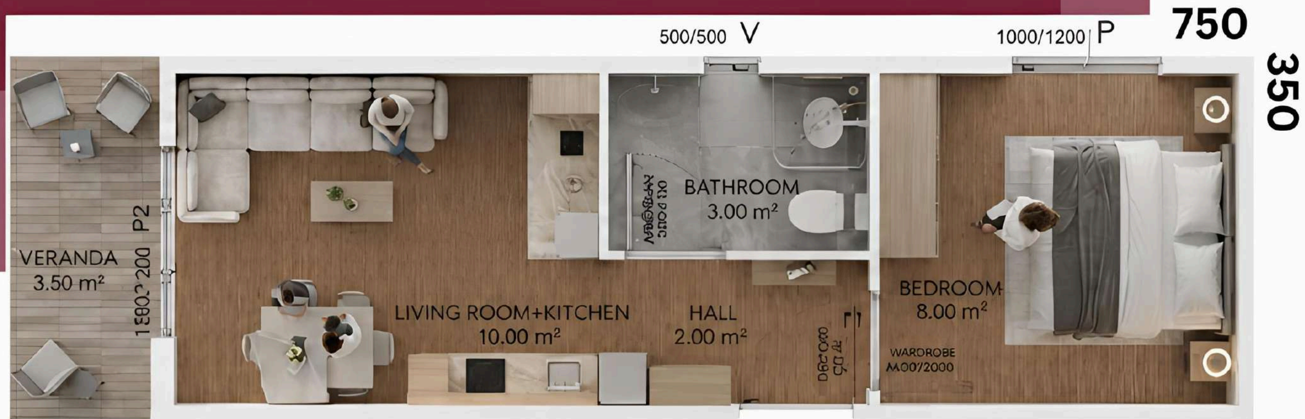
26.5 m 2 SINGLE-STORY PREFABRICATED HOUSE PLAN
