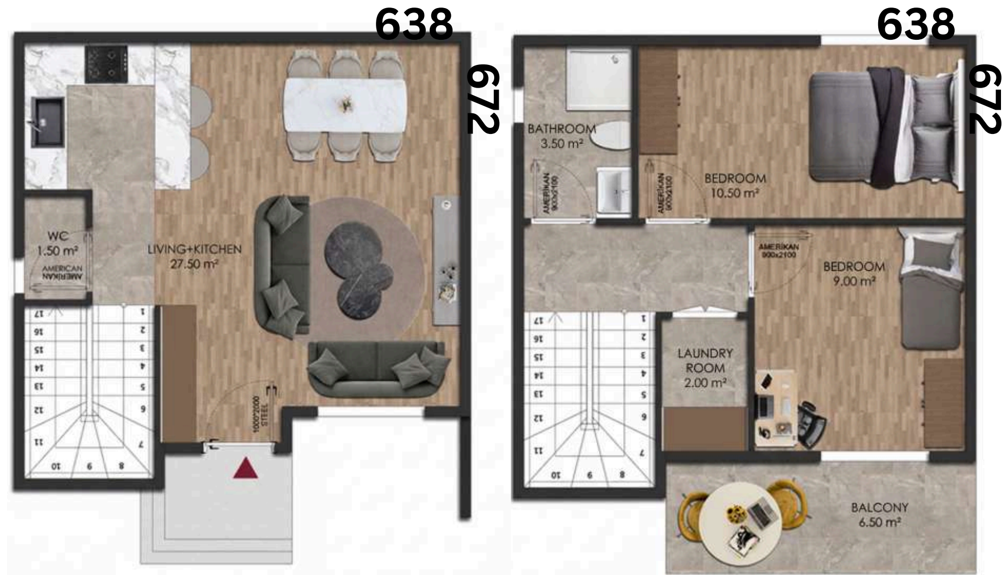
PLAN OF A 60.5m 2 TWO-STORY PREFABRICATED HOUSE
