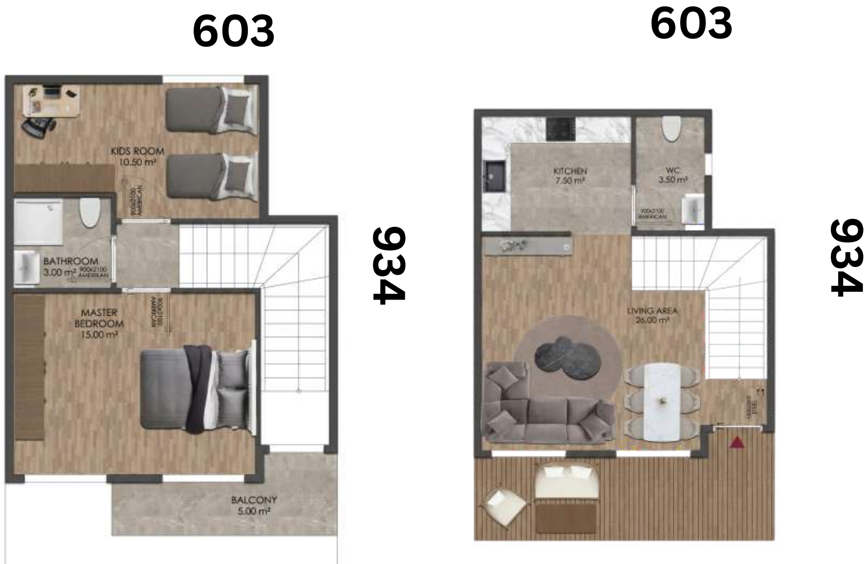
PLAN OF A 64m2 TWO-STORY PREFABRICATED HOUSE
